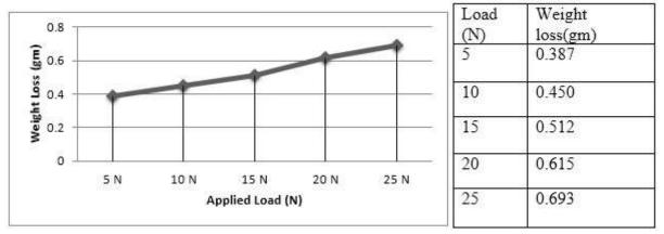
It can be observed from the above figure that as the applied load increases, the wear rate (weight loss) also increases. Also as the position changes from horizontal to vertical, the wear mass decreases due to change in orientation of forces.
